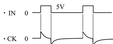
The capacitor coupling allows reset pulses to be supplied intermittently from the RESET pin whether the input level (IN) is high or low.
