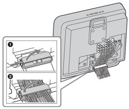
I • The hook of the cable holder can be opened from either sides depending on attaching position.
