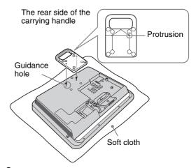
**3** Fix the carrying handle to the TV securely with the four screws (supplied) for the carrying handle.
