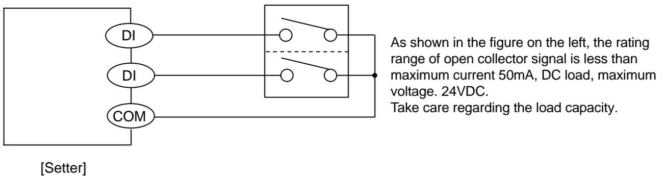
Various external signal inputs (DI) operate by short circuiting specified external signal input terminal and common (COM) terminal. Operation by switch and relay is a general method however operation by open collector output signal of peripheral device is also possible.
