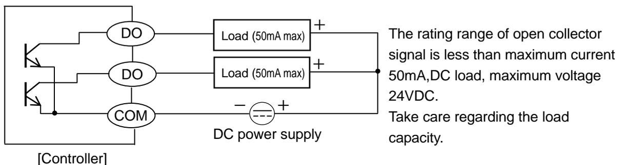
Various external signal outputs (DO) are output using open collector signals. If AC power supply is applied or load other than the rating range is applied, the controller may get out of order or its performance may deteriorate remarkably or it may malfunction.
