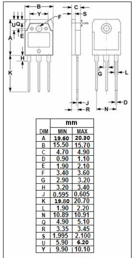
**isc Silicon NPN Power Transistor**
