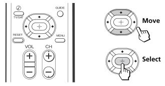
To navigate on the on-screen menus, use the "arrow" buttons  $(\diamondsuit, \heartsuit, \diamondsuit, \diamondsuit)$  to move the cursor. Pressing these arrows will cause the cursor to move in the corresponding direction. Pressing center button  $(\textcircled{\Rightarrow})$  will allow you to select an option.
