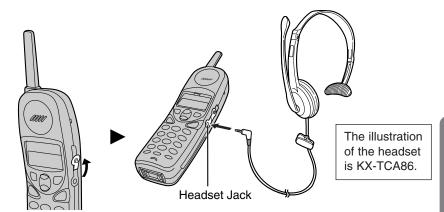
When an optional headset is connected to the handset, make sure to use the headset to talk with the caller. If you want to have a normal cordless phone conversation, disconnect the headset.
