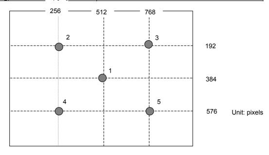
Note 1: Average brightness is the average of brightness value at location 1 to 5 with all (C) Copyright Acer Display Technology, Inc.
