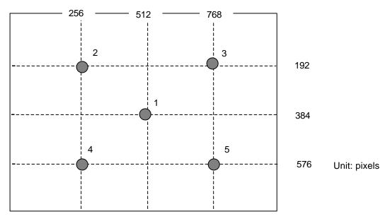
Note 1: Average brightness is the average of brightness value at location 1 to 5 with all pixels displaying white.
