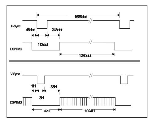
Note :1280X1024 at 75 Hz (VESA STANDARD), Horizontal line rate :13.02us, Dot clock :135MHz.
