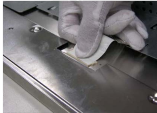
Pull out the LVDS cable
