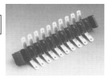
A ten way barrier type terminal block which can easily be sub-divided if required. It has two rows of solder or solderless snap-on connextors (2.8mm x 0.61mm).
