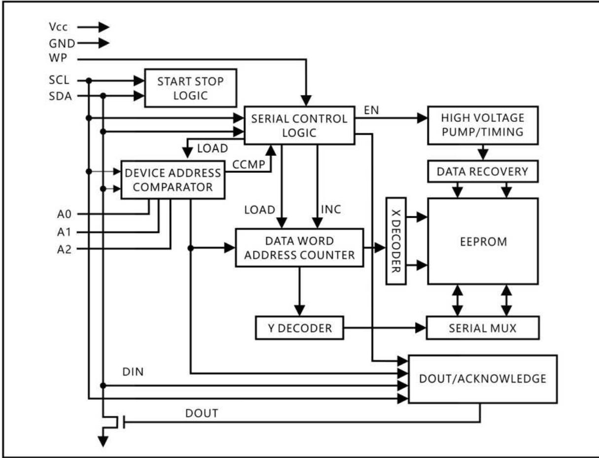
**DEVICE/PAGE ADDRESSES (A2, A1 and A0):** The A2, A1 and A0 pins are device address inputs that are hard wire for the L24C64A. Eight 64K devices may be addressed on a single bus system (device addressing is discussed in detail under the Device Addressing section).
