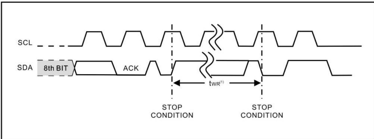
Note: 1. The write cycle time  $t_{WR}$  is the time from a valid stop condition of a write sequence to the end of the internal clear/write cycle.
