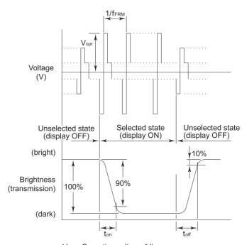
$\begin{array}{l} V_{\text{opr}}: \text{Operating voltage (V)} \\ f_{\text{FRM}}: \text{Frame frequency (Hz)} \\ t_{\text{on}}: \text{Response time (rise) (ms)} \\ t_{\text{off}}: \text{Response time (fall) (ms)} \end{array}$
