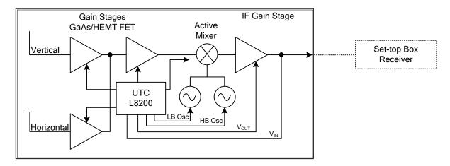
Polarization and band switching on the UTC **L8200** uses the standard 13~17V and 22kHz as defined by Astra. The exception is that the devices voltage detector has a much tighter tolerance than required to increase field reliability.
