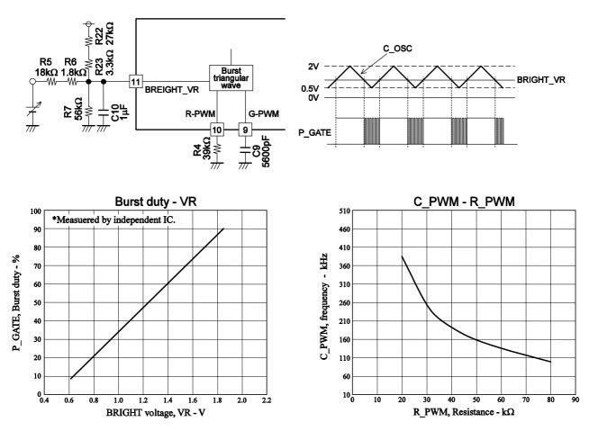
\* The above graph is based on measurements for the independent IC.
