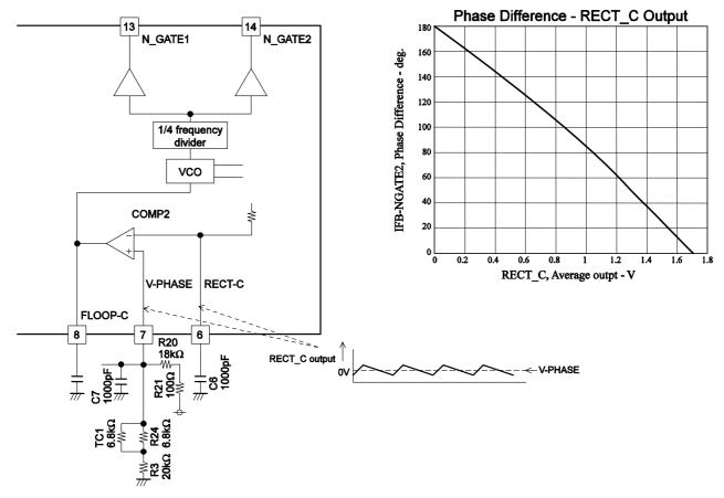
\* The above graph is based on measurements for the IC in isolation. Actual phase difference adjustment requires connection to the piezoelectric transformer.
