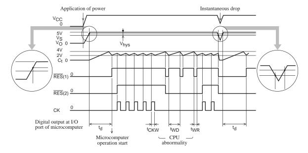
Note: Edge-triggered at the point indicated by the arrow of CK signal.
