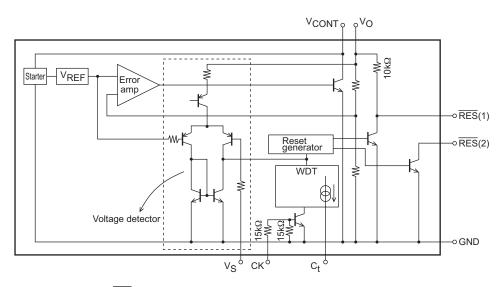
$\overline{RES}(1)$ : Contains a pull-up resistor of  $10k\Omega$ .
