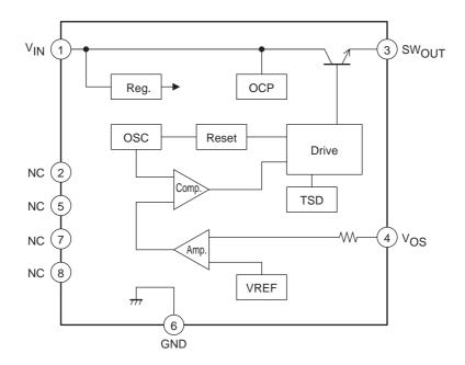
Note: Since the NC pins are not connected within the IC package, they can be used as connection points.
