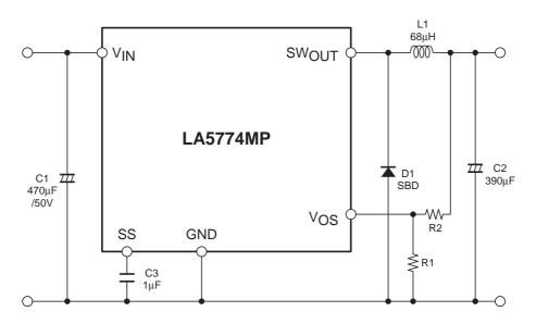
Notes: C3 is for the soft start function. Delete C3 and keep the SS pin open when the soft start function is not necessary.
