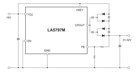
Note: The IC is made active when the EN pin is pulled down to GND. The charge pump operation is stopped when the EN pin is pulled up to  $V_{IN}$ .
