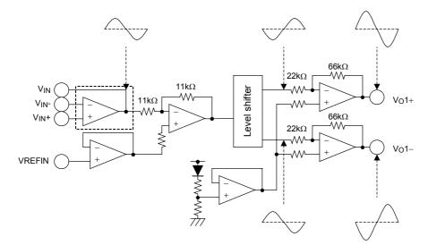
Note \*: Only channel 1 has an added input operational amplifier.
