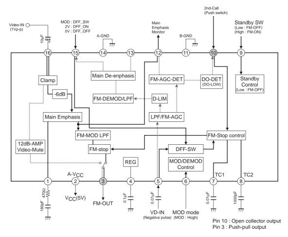
Application Circuit Example2 Demodulation (Monitor)
