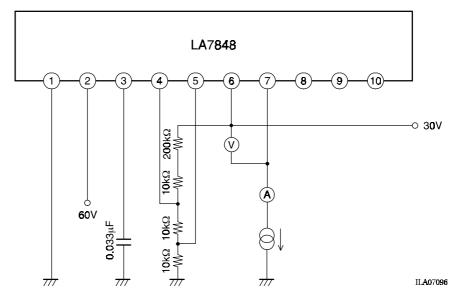
In the circuit in figure 4 with the output from pin 7 absorbed by an electronic load, read the value shown by the voltage meter (V) when the current meter (A) reads 1.1A.
