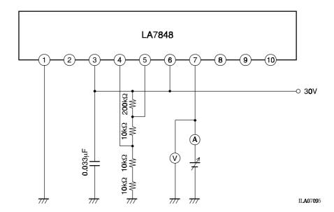
In the circuit in figure 3, read the value shown by the voltage meter (V) when the current meter (A) reads 20mA.
