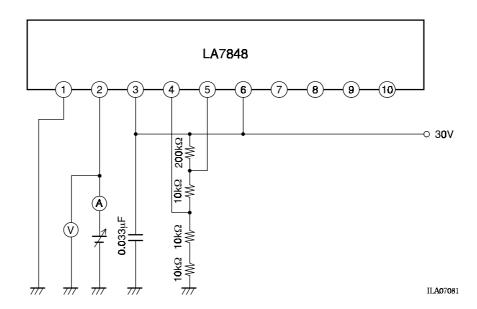
In the circuit in figure 1, read the value shown by the voltage meter (V) when the current meter (A) reads 1.1A.
