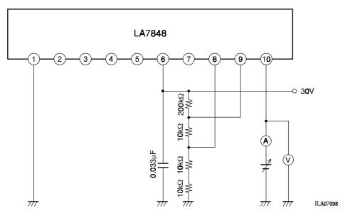
In the circuit in figure 6, read the value shown by the voltage meter (V) when the current meter (A) reads 500mA.
