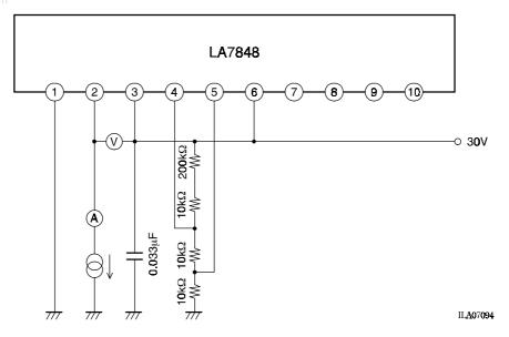
In the circuit in figure 2 with the output from pin 2 absorbed by an electronic load and read the value shown by the voltage meter (V) when the current meter (A) reads 1.1A.
