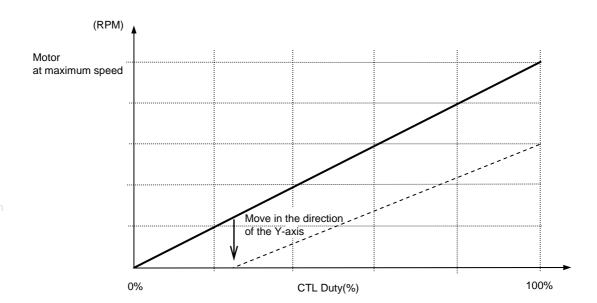
(Example) In the case where the characteristics change from ones with the origin point (0%, 0 rpm) to ones where the speed at a duty ratio of 25% becomes 0 rpm:
