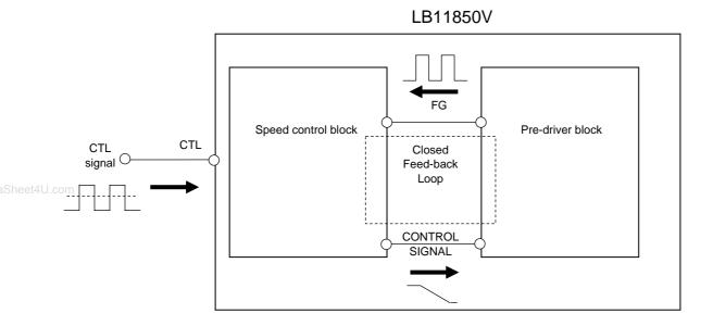
The operation inside the IC is as follows. Pulse signals are created from the edges of the FG signals as shown in the figure below, and a waveform with a pulse width which is determined by the CR time constants and which uses these edges as a reference is generated by a one-shot multivibrator.
