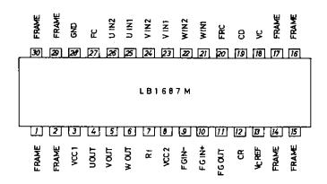
Note: All FRAME pins are connected to GND.
