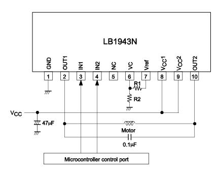
Note: Microcontroller output ports must be CMOS outputs and must be used in the high, low, or open state.
