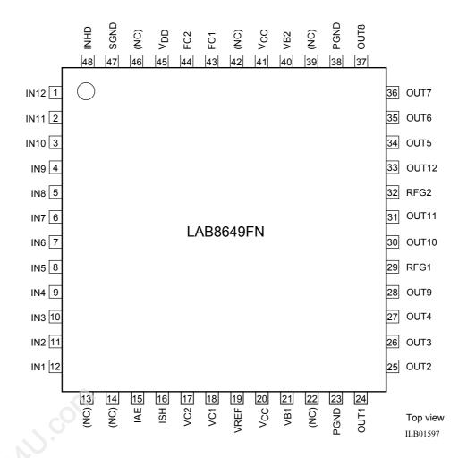
(Note) PGND is connected with both 2 pins.
