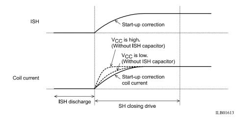
The ISH pin input voltage is set with the decay time constant to be larger than the coil decay time constant by using the external CR and the start-up correction occurs with respect to the coil wave.
