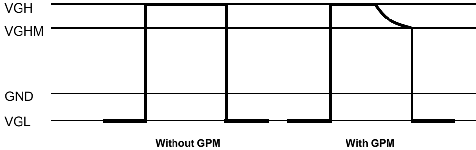
FIG. 1 Gate Output Wave form without GPM and with GPM
