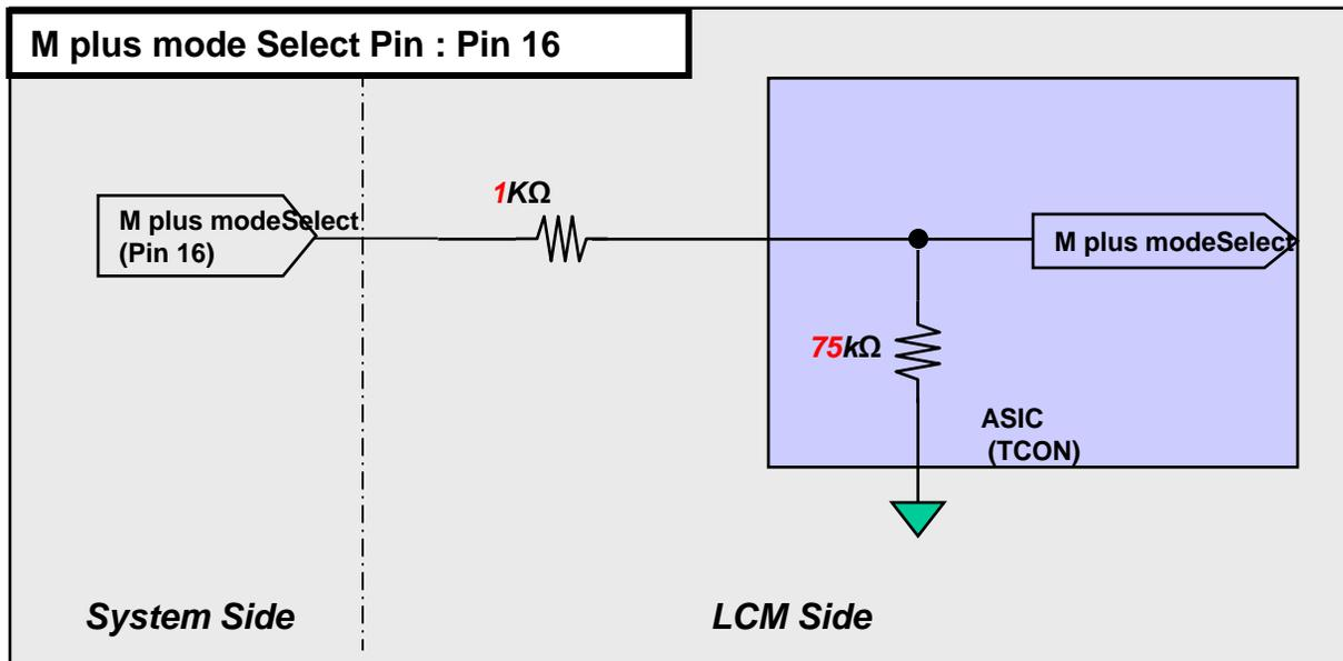
2) Circuit Block Diagram of M plus Enable pin
