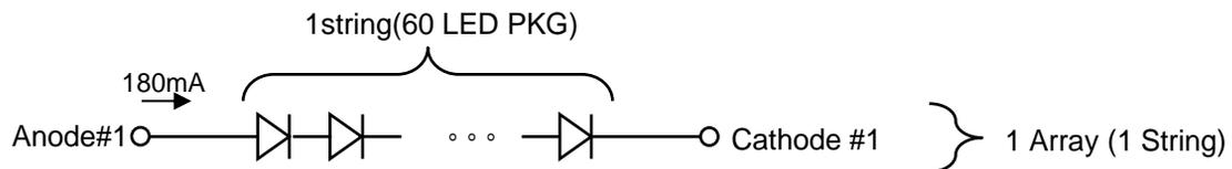
4. The forward voltage( $V_F$ ) of LED array depends on ambient temperature (Appendix-V)
