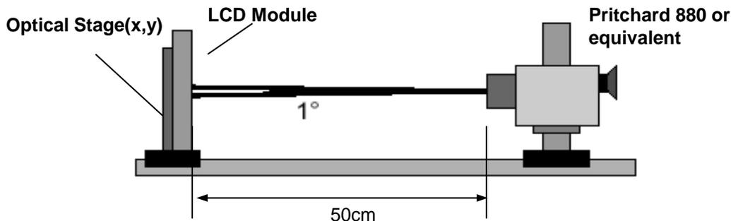
FIG. 6 Optical Characteristic Measurement Equipment and Method
