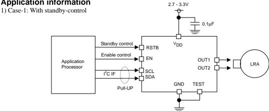
Note) When SDA&SCL signal voltages are different from VDD, even if the RSTB pin is set to Low, the IO leak current flows. ex) In case of VDD=3.0V & SDA=SCL=1.8V, the current consumption is about 100µA(typ).
