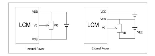
$V_{DD^{\sim}}V_0$ : LCD Driving voltage
