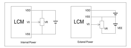
$V_{DD-}V_0$ : LCD Driving voltage VR: 10k~20k
