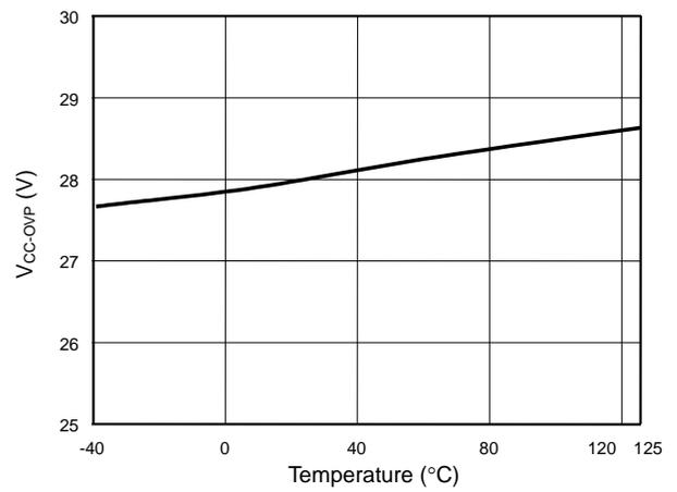
Fig. 10 V<sub>VCC-OVP</sub> vs. Temperature
