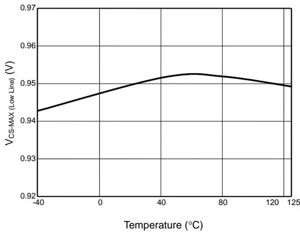
Fig. 9 V<sub>CSMAX</sub> (Low Line) vs. Temperature
