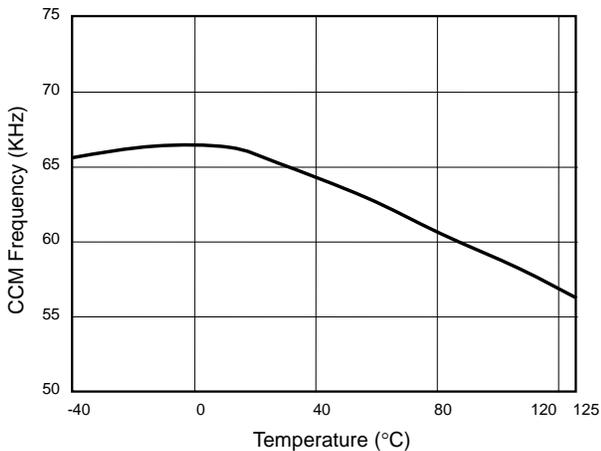
Fig. 5 CCM Frequency (High Line) vs. Temperature
