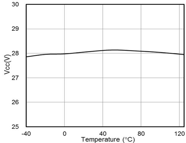
Fig. 6 Vcc OVP Level vs. Temperature
