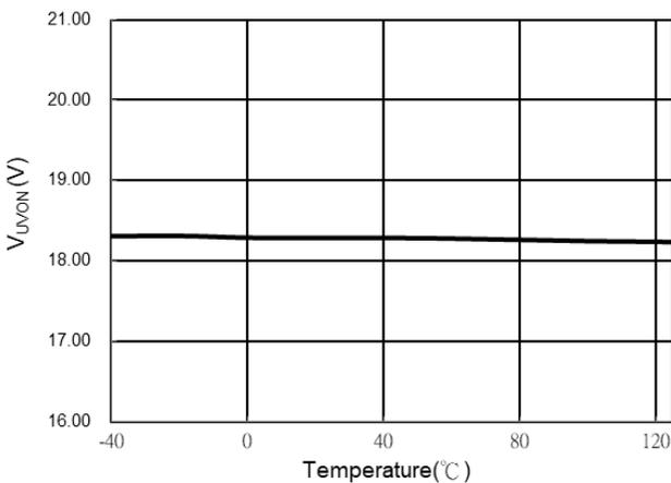
Fig.5 V<sub>UVON</sub> VS. Temperature
