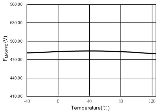
Fig. 18  $F_{MAXPFC}$  VS. Temperature
