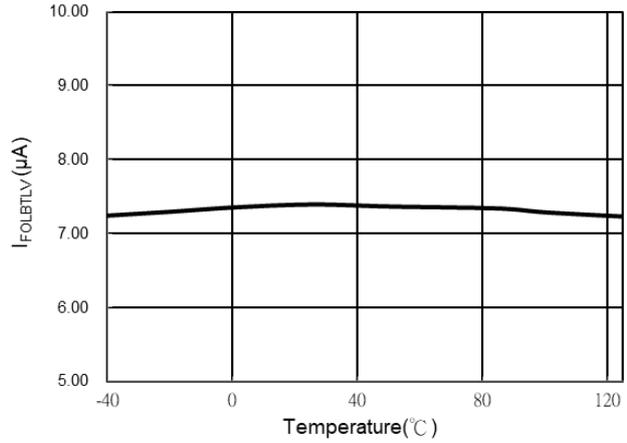
Fig. 14  $I_{FOLBTLV}$  VS. Temperature
