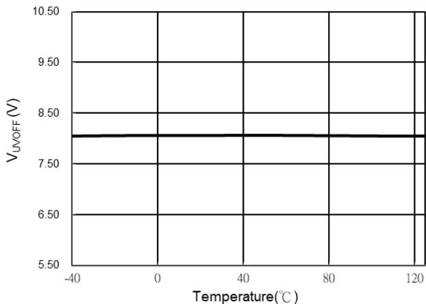
Fig.6 V<sub>UVOFF</sub> VS. Temperature
