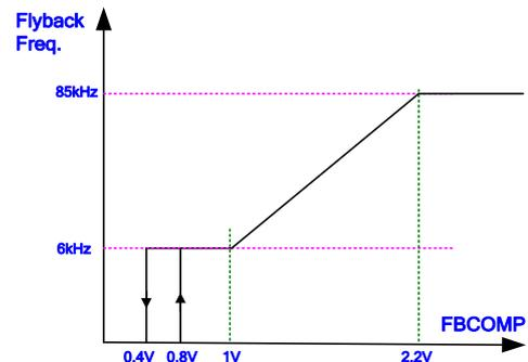
Fig. 27 Max. Frequency Limit of Flyback
