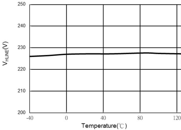
Fig.3 V<sub>HLINE</sub> VS. Temperature
