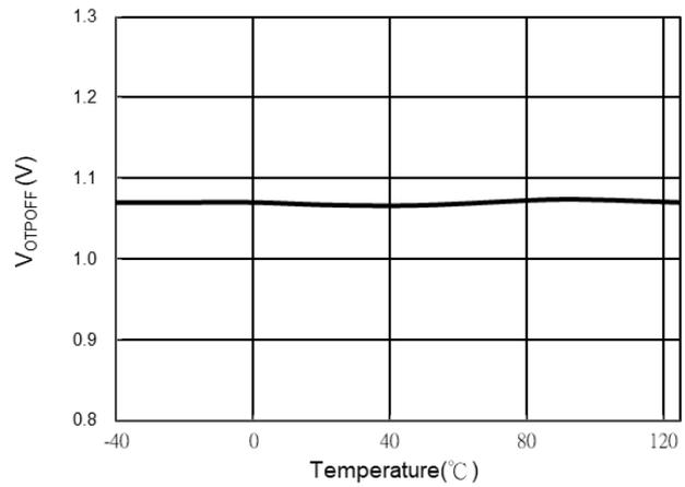
Fig. 10 V\_OTPOFF VS. Temperature
