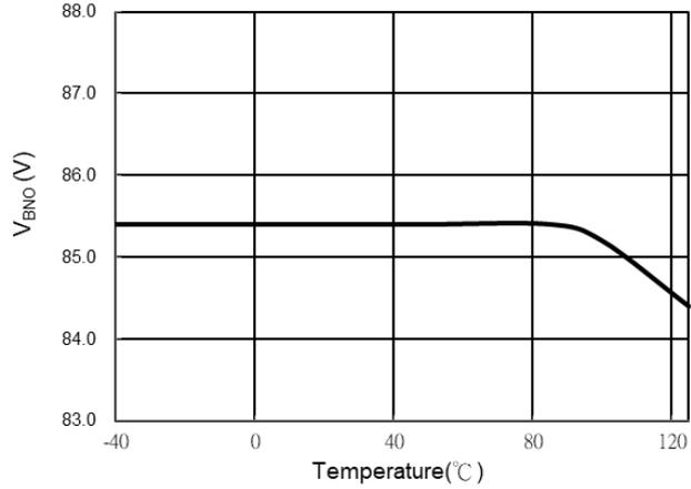
Fig.2 V<sub>BN0</sub> VS. Temperature
