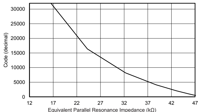
Figure 10. Transfer Characteristics of LDC1000-Q1 With R_{P\_MIN} = 16.160 \text{ k}\Omega and R_{P\_MAX} = 48.481 \text{ k}\Omega
