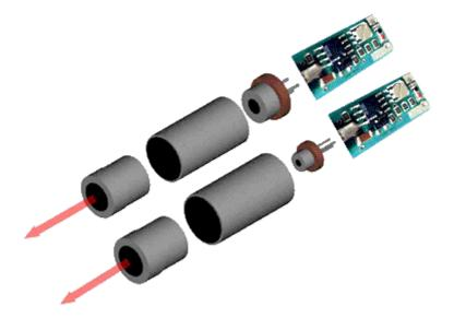
To get the LD mounted, you need to glue it into the holding fixture.
