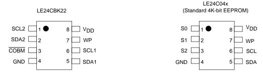
Pin 3 of standard 4K-bit EEPROM products is assigned a slave pin (S2), but Pin 3 of the LE24CBK22 is assigned the COBM pin. Combined mode is entered by setting the COBM pin low. In combined mode, the state of the SCL2 pin and SDA2 pin is "don't care" (may be either high, low, or open).
