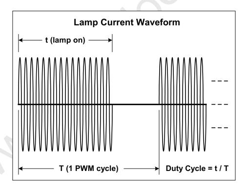
The lamp current waveform with the PWM circuit set at less than 100%
