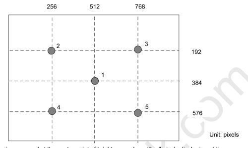
Note 1: Brightness is measured at the center point of brightness value with all pixels displaying white.
