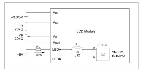
\* VR is for LCD contrast adjusting, VDD-VO is around 22.6V
