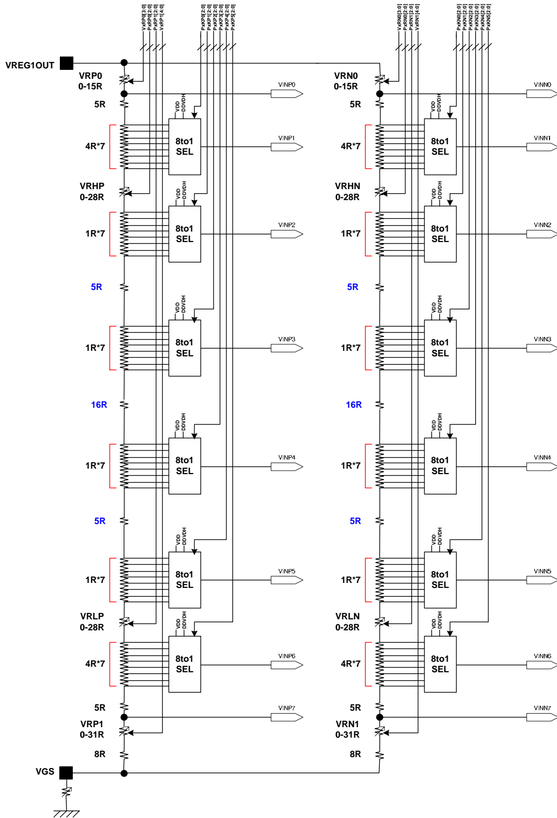
Figure 67 Ladder resistor units and 8-to-1 selectors (IPS=0)
