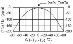
The curve shown above accounts for resonator contribution only and does not include oscillator temperature characteristics.
