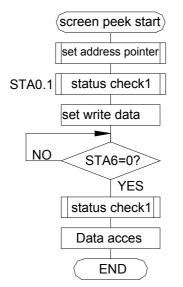
Note: this command is available when hardware column number and software column number are the same. Hardware column number is related to MD2 and MD3 setting. Software column number is related to ser text area and set graphic area command.
