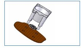
Do not look directly into the high-power LED light source. The high intensity beam could cause irreversible damage to your eyes. Figure 5 How to assemble lens (holder), ACULED and substrate (heat sink) in principle.
