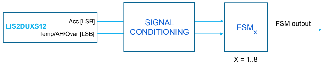
Figure 12. State machine in the LIS2DUXS12
