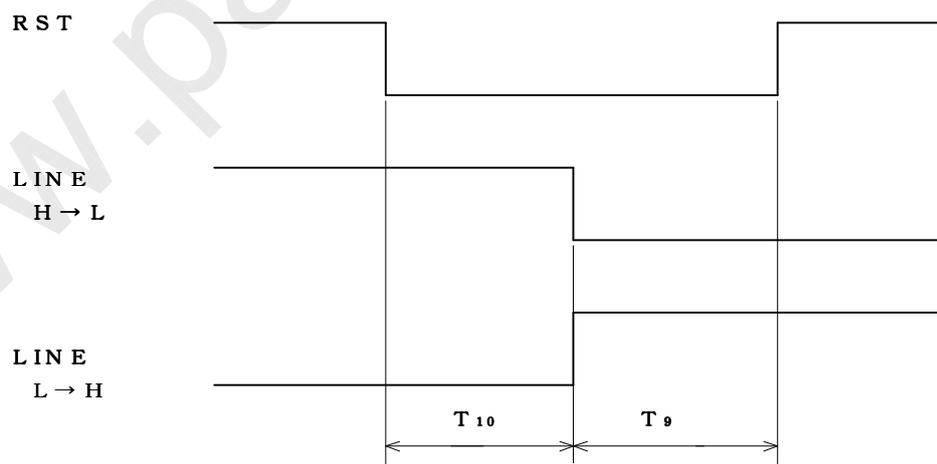
Note)  $T_9, T_{10} \geq 8\text{ms}$  shall be kept.
