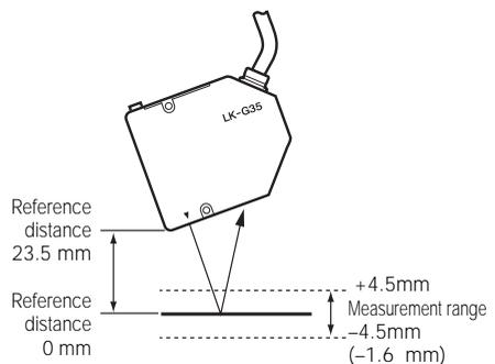
\* The value inside the parentheses ( ) is when the sampling rate is 20  $\mu$ s.
