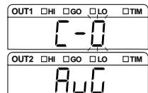
4 Press the **ENT** key, and specify the number of times of moving average with the **▲** key.
