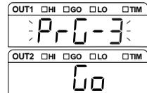
**3** Press the **ENT** key to initialize. Press the **SET** key to return to the measurement state.
