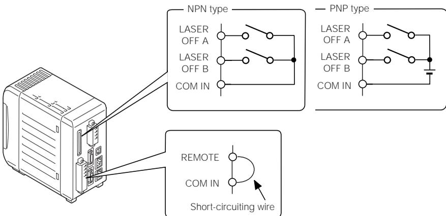
\* The laser remote interlock connector is delivered with the wire for short-circuiting installed.
