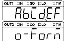
Set the output form of the tolerance comparator.
