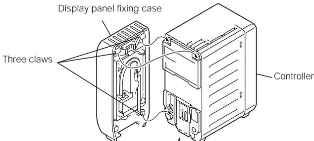
**4** Install the display panel fixing case along the groove on the controller.
