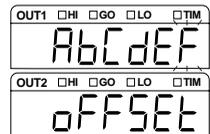
**3 Press the **ENT** key, and set the offset value with the **▶** and **▲** keys.**
