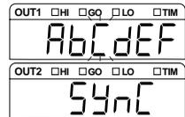
Set the synchronization/asynchronization of the external timing.
