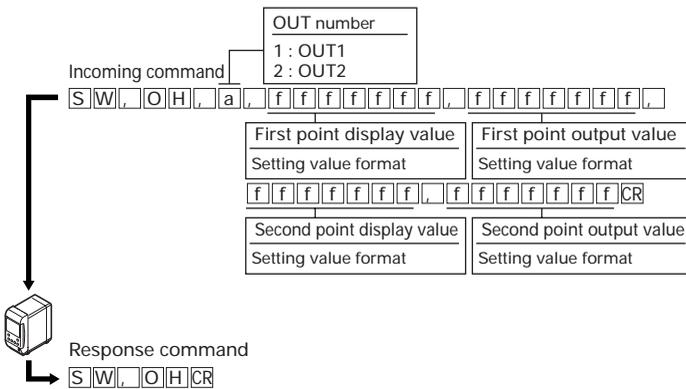
\* Set the voltage value in mV for the setting value format of the output value.
