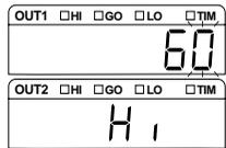
5 Press the **ENT** key, and set the value for the lower limit with the **▶** and **▲** keys.
