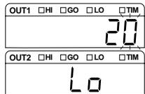
6 Press the **ENT** key to register the setting. Press the **SET** key to return to the measurement state.
