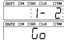
**7** Press the **ENT** key to perform copying. Press the **SET** key to return to the measurement state.
