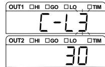
5 Press the **ENT** key to register the setting. Press the **SET** key to return to the measurement state.
