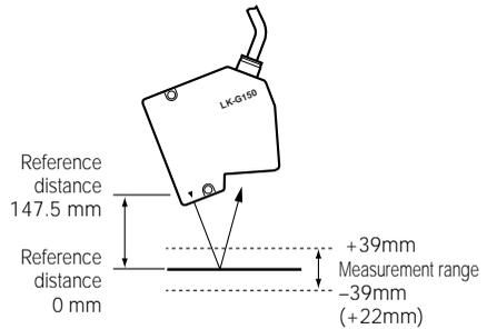
\* The value inside the parentheses ( ) is when the sampling rate is 20  $\mu$ s. Note that the measurement range narrows, disabling measurements at the reference position.
