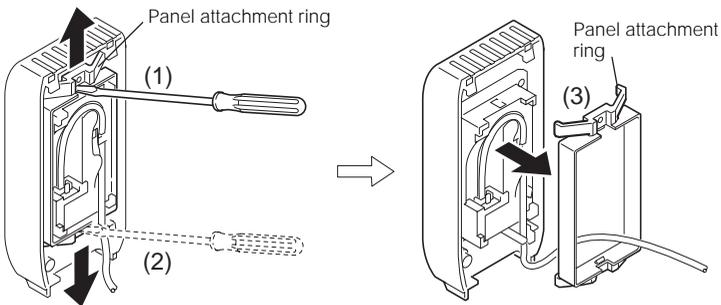
**5** Remove the display panel from the display panel fixing case.
