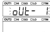
2 Press the **ENT** key, and select the function "C" with the **▶** key.
