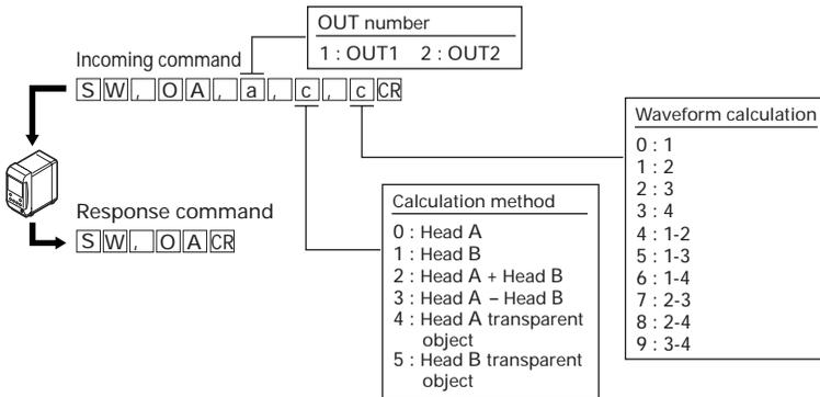
\* Even when specifying a value from 0 to 3 for the calculation method, specify dummy data for the calculation between waveforms.
