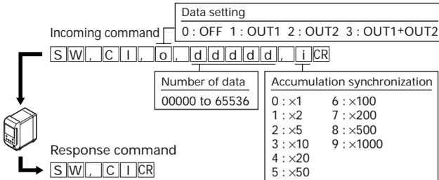
Sampling rate, mutual interference prevention, timing synchronization, comparator output form, and strobe time
