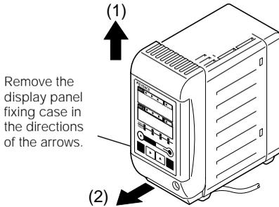
**4** While pushing (1) and (2) outward in this order, push the display panel to remove the panel attachment ring.
