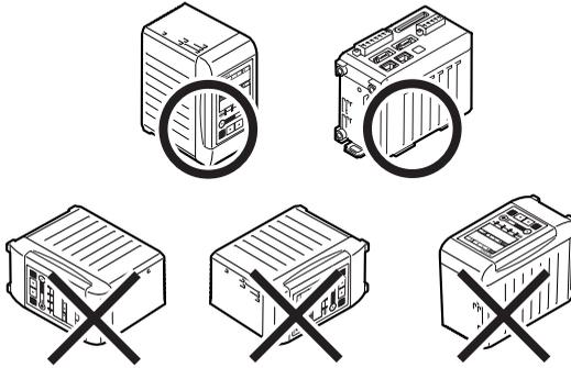
Be sure to leave 30 mm of clearance or more above the controller, and 10 mm or more on each side.
