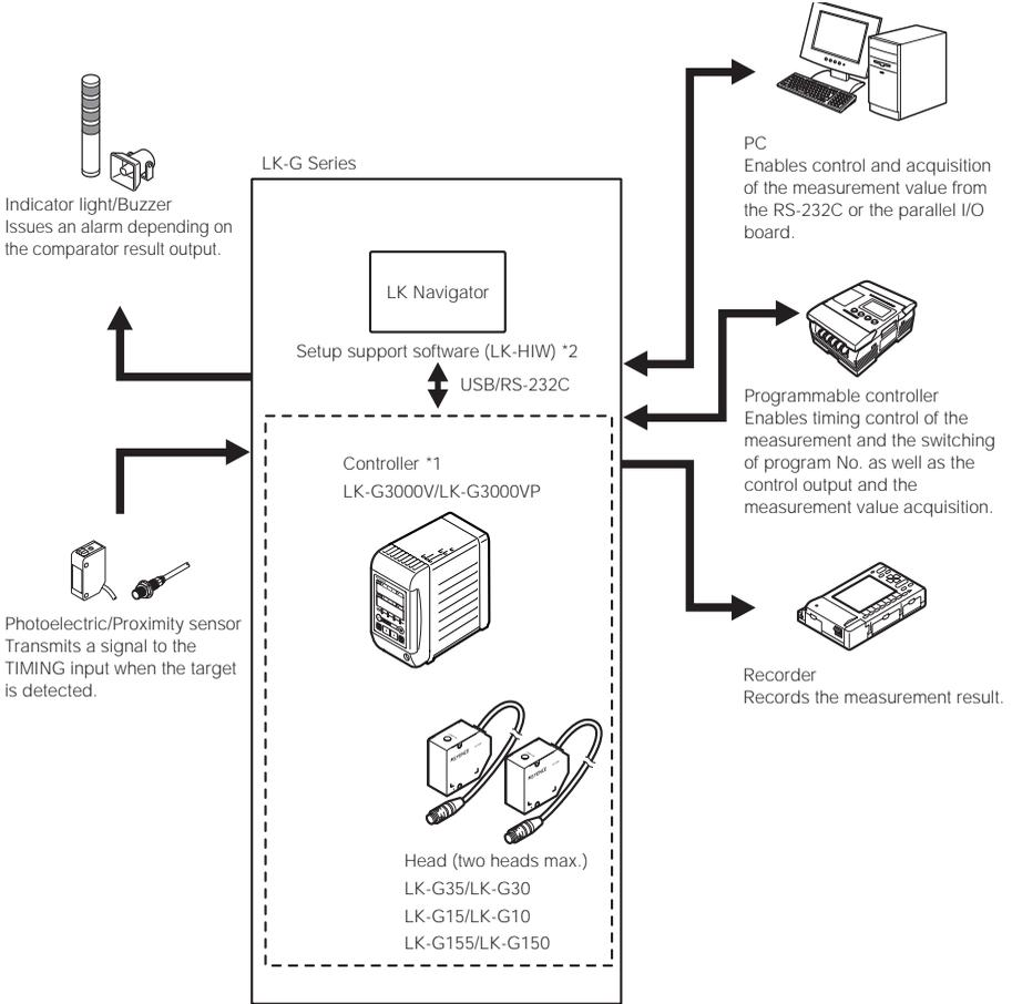
\*1: The controller (LK-G3001V/LK-G3001VP) can be separated into the display panel and the controller main unit. You can also purchase them separately.
