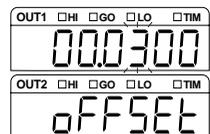
**4 Press the **ENT** key to register the setting. Press the **SET** key to return to the measurement state.**
