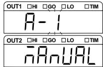
4 Press the **ENT** key, and set the value for the higher limit with the **▶** and **▲** keys.
