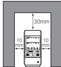
When installing the controllers side-by-side, make sure there is a clearance of 10 mm or more between the controllers and 30 mm or more of clearance above them.
