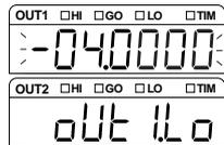
**4 Confirm the data by pressing the ENT key, and press the SET key to return to the measurement state.**
