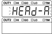
2 Press the **ENT** key, and select the function "A" with the **▶** key.
