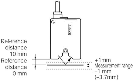
\* The value inside the parentheses ( ) is when the sampling rate is 20  $\mu$ s.
