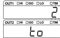
**6** Press the **ENT** key to check the program Nos. of the copy source and destination.
