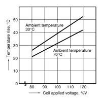
3. Ambient temperature characteristics Contact current: 5 A
