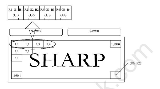
[Note] Scan direction is setting for using S-PWBs' side up.
