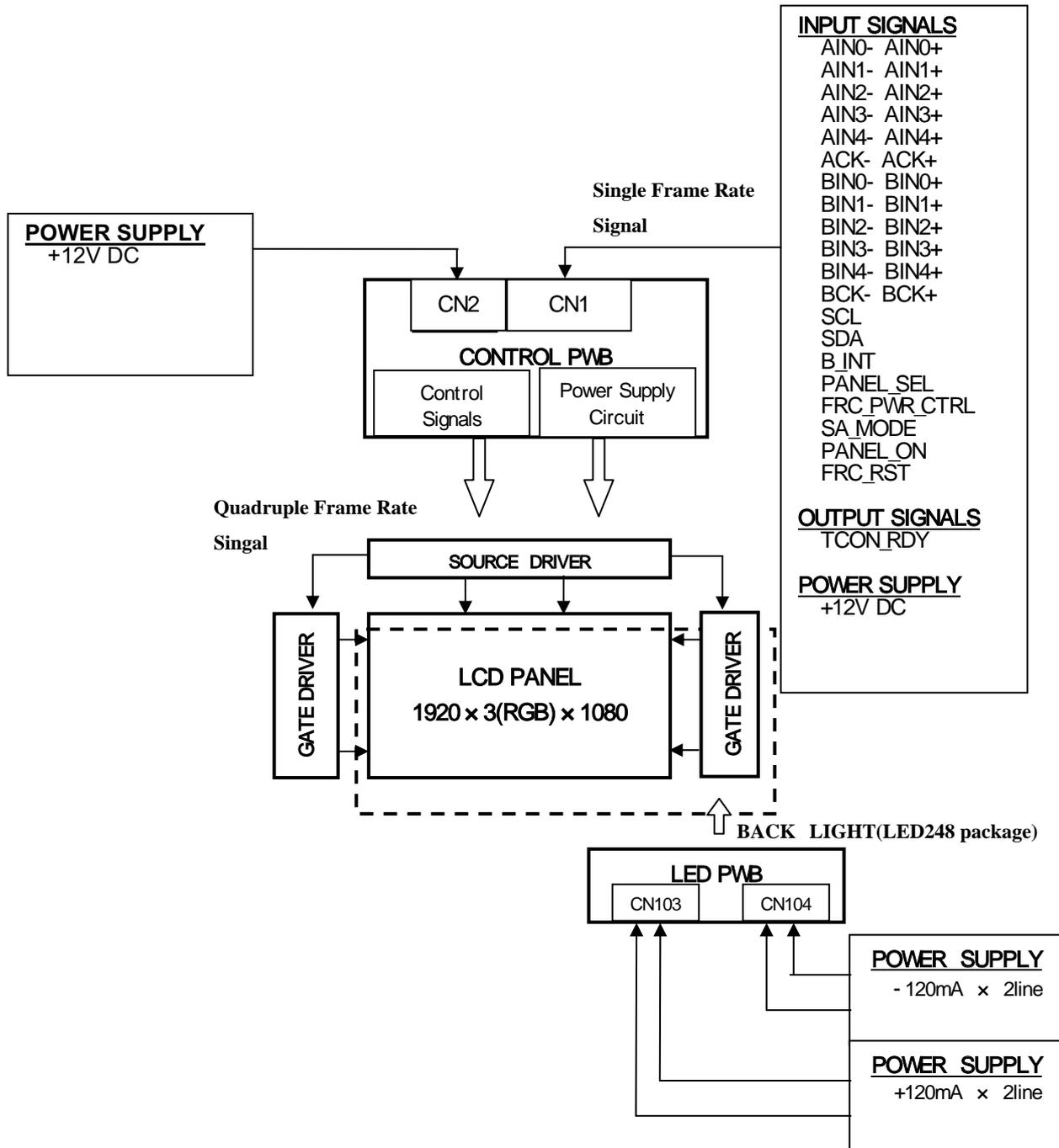
Fig.3 Interface block diagram
