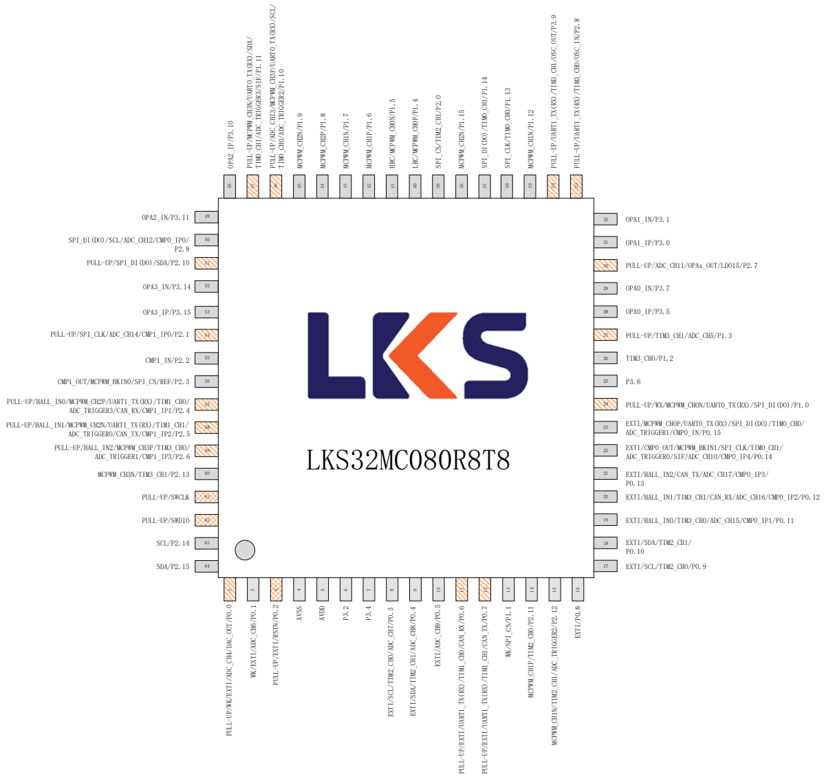
Fig. 3-1 LKS32MC080R8T8(B) Pin Assignment
